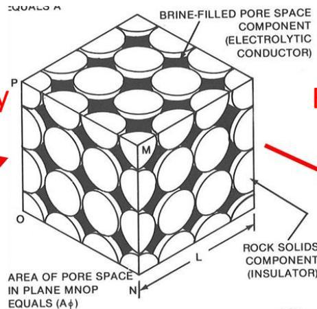
Electric charges are only conducted through tortuous paths of brine filled pore space
